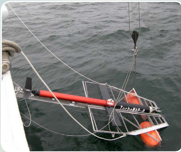
The TurboMap-G (H Yamazaki, Japan) device allows us to understand the small-scale physical hydrodynamics that control the aggregation of toxic microalgae in thin layers in the water column. Photo: H. Yamazaki.
