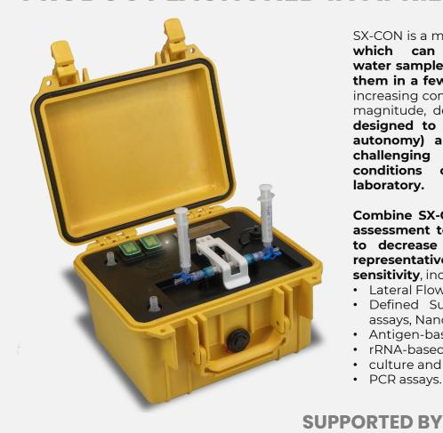
SX-CON is a microorganism concentrator module which can rapidly filtrate large volume of water samples (in the order of litres) and elute them in a few millilitres reservoir, providing an increasing concentration factor of some orders of magnitude, depending on the application. It is designed to be portable (with large battery autonomy) and robust to use in the most challenging outdoors' environmental conditions or simply operating in the laboratory.
